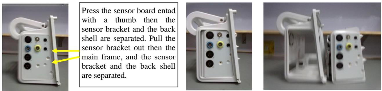
Press the sensor board end with a thumb then the sensor bracket and the back shell are separated. Pull the sensor bracket out then the main frame, and the sensor bracket and the back shell are separated.
