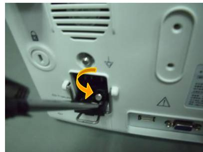
4. Replace the old fuse with a new one that is supplied by EDAN or with the same specifications. (Dimensions:  $\Phi 5\text{mm} \times 20\text{mm}$ ; model: T3.15AH 250VP)
