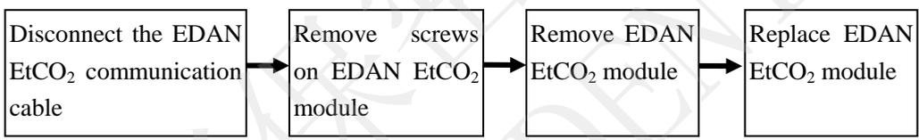
Assemble the EDAN EtCO<sub>2</sub> module in the reversed order.
