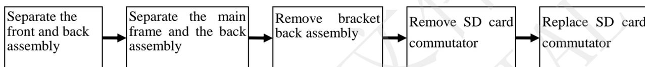
Assemble the SD card commutator in the reversed order. For detailed information, please refer to section 8.5.5.
