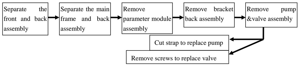
Assemble the pump&valve in the reversed order.
