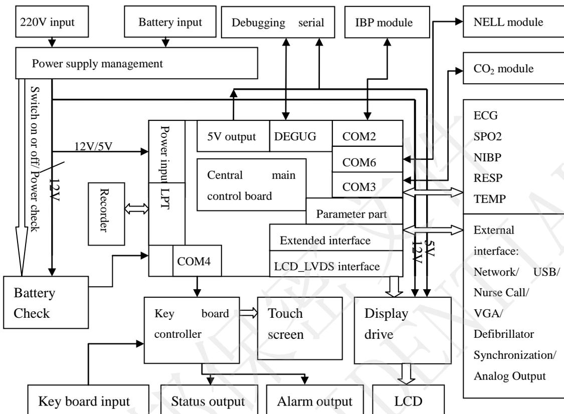
Figure 6-1 iM50/M50 System Principle Block Diagram
