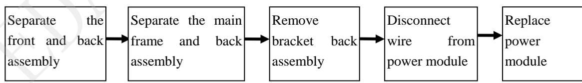
Assemble the power module in the reversed order.
