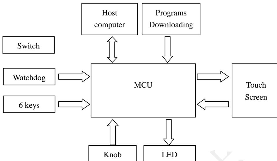
Figure 6-2 Key Board Hardware Block Diagram
