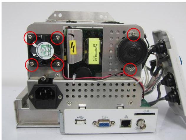
Figure 8-7 Replacing the Fan and the Speaker
