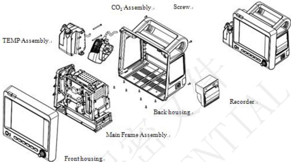
Figure 8-1 Main Unit Structure Block Diagram
