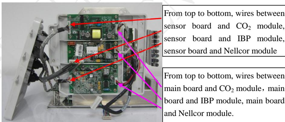
Figure 8-8 Replacing CO<sub>2</sub> Module, IBP Module and Nellcor Module
