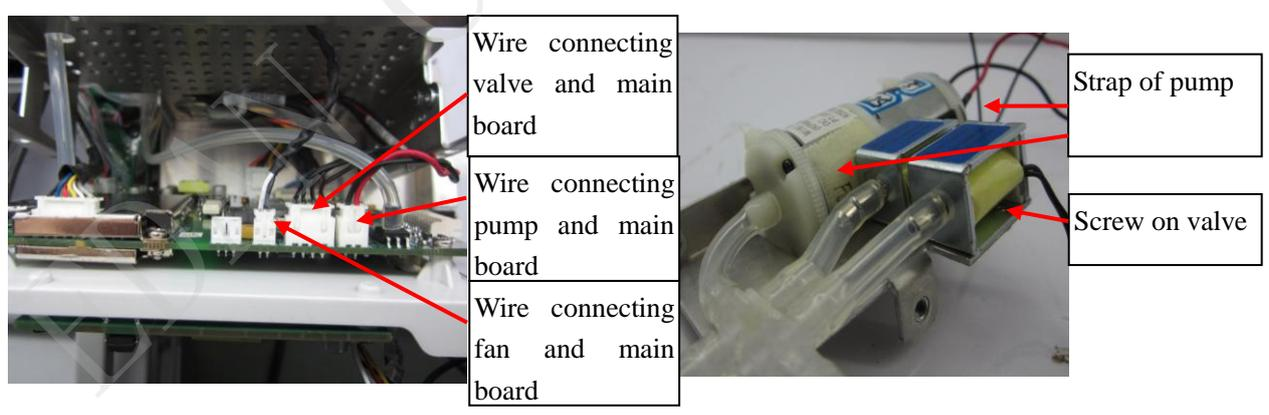
Figure 8-10 Replacing Pump&Valve
