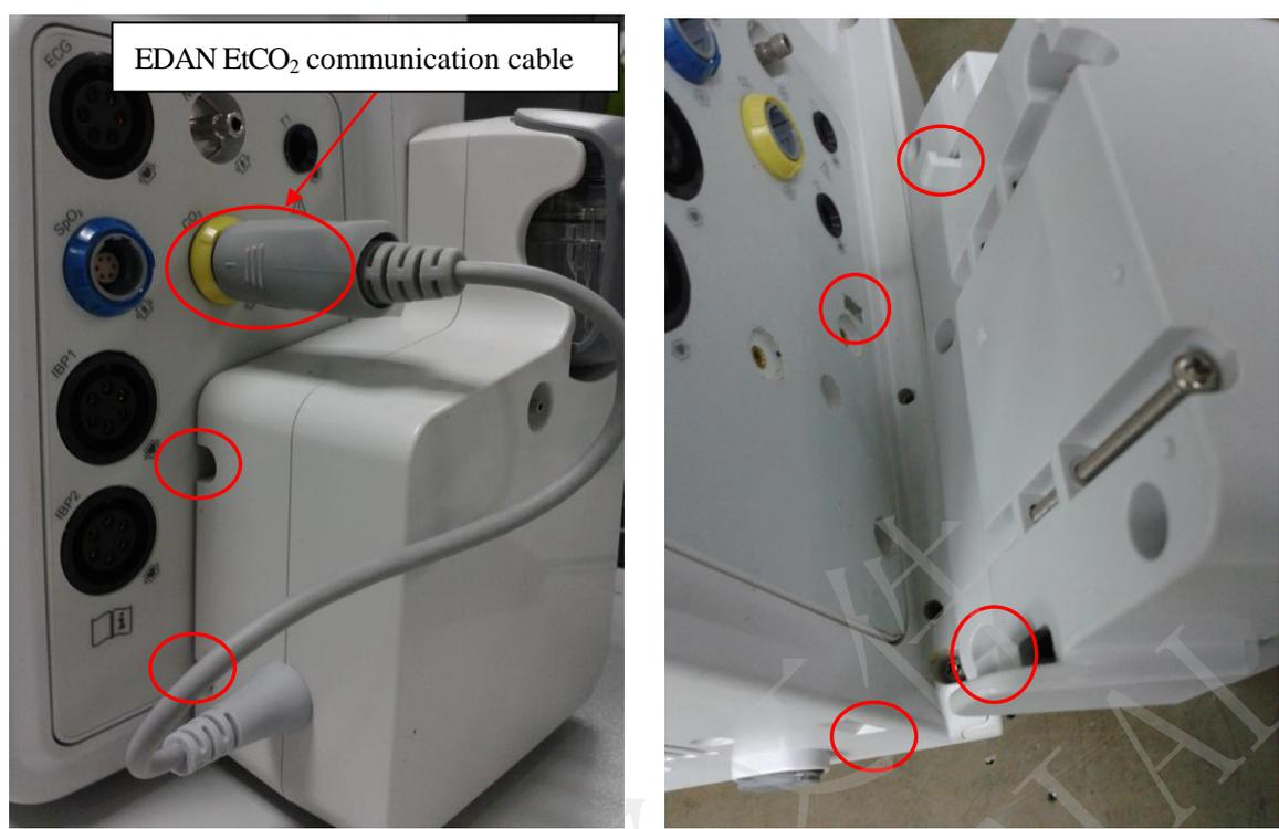
Figure 8-13 Replacing EDAN EtCO<sub>2</sub> Module
