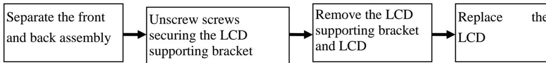
Assemble the LCD in the reversed order. Please refer to the diagram on the section 8.4.1.
