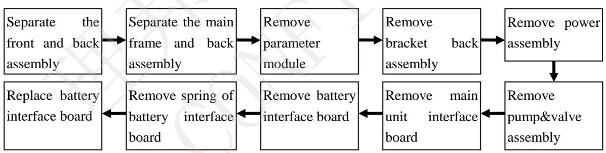
Assemble the battery interface board in the reversed order.
